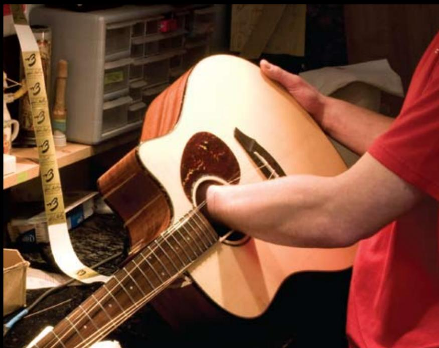
Left, A Breedlove craftsman adjusts the bridge truss system at the beginning of the quality control process.
